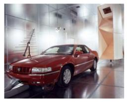
ETS-Lindgren's SMART<sup>™</sup> (Statistical Mode Averaging Reverberation Test-Site) Chambers use the latest developments in proven reverberation technology and experienced chamber design and construction, to create a suitable electromagnetic environment (EME) for immunity, emissions and shielding effectiveness testing.Compared with other test methods, SMART chambers offer the advantages of lower cost, higher field-to-input power ratios, and the ability to accept large test systems.
